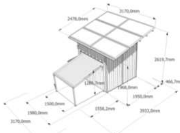
Fig. 2 – OGB scheme: Technologies mix and dimension after complete installation.
