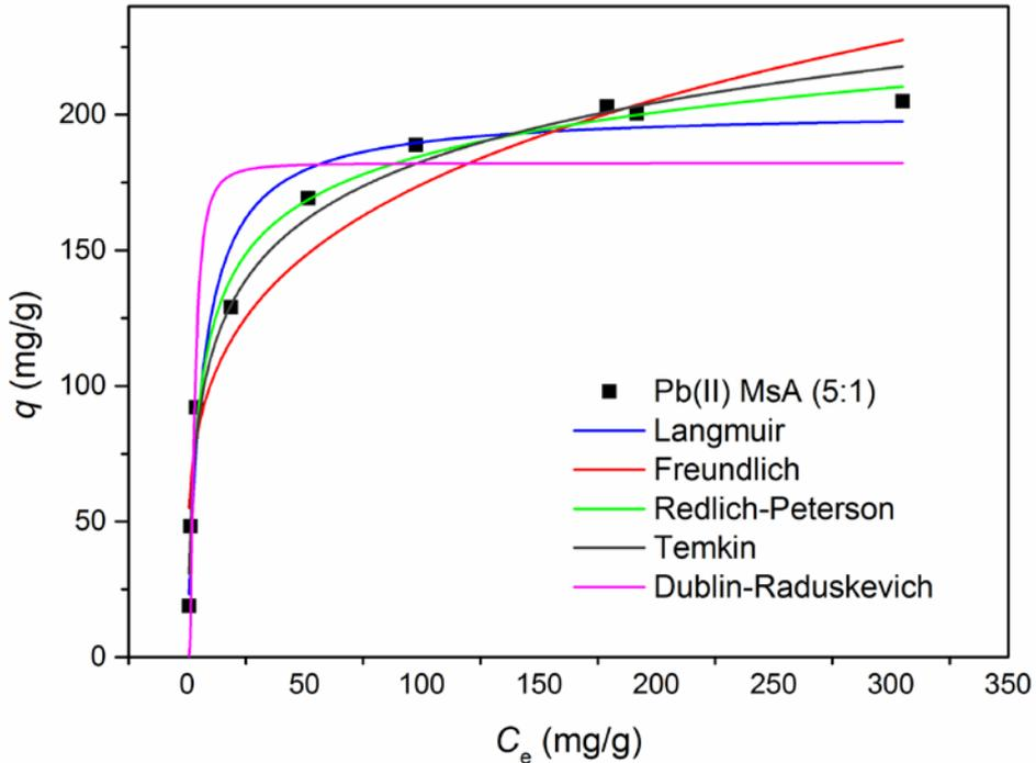
Figure 3 Lead sorption isotherms of MsA(5:1) bead at pH 5 (initial concentrations: 0.2 - 4 mmol/l;  $m = 0.1$  g; pH 5; agitation rate 200 rpm).
