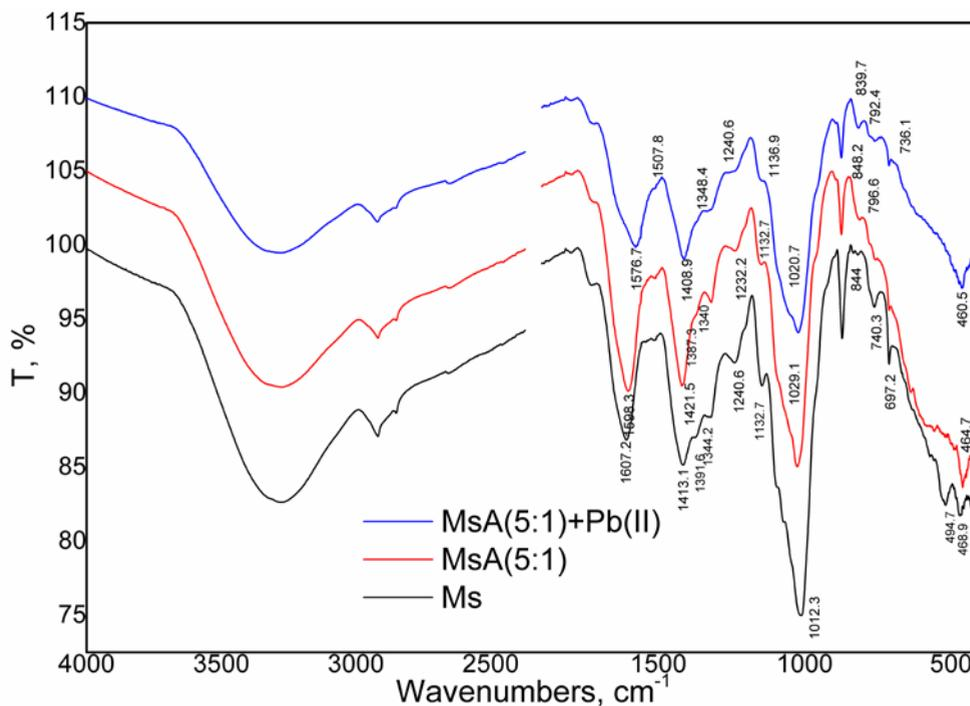
**Figure 2.** FT-IR spectra: *M. spicatum* (washed, particle size less than 0.2 mm), MsA (5:1) before and after Pb(II) biosorption (contact time 24 h, pH=5, Pb(II) initial conc. 3 mmol/l, agitation rate 200 rpm)
