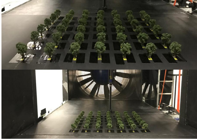
Figure 3. Placement of grid olive grove over flat terrain inside the IISTA Atmospheric Boundary Layer Wind Tunnel.
