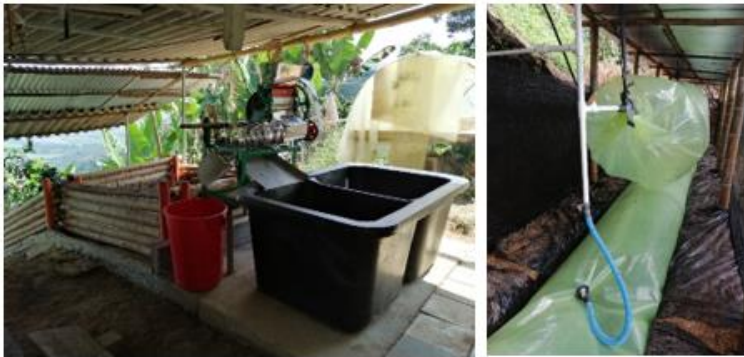
Photo 1 and 2. green coffee production system and mixed anaerobic biodigester for the management of coffee and pig farming waste.
