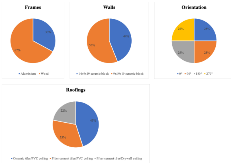
Figure 8: Frequency of occurrence of construction components and solar orientation of buildings with lower impact in damage categories
